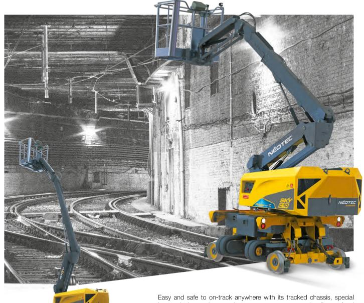
Easy and safe to on-track anywhere with its tracked chassis, special boom design to bypass the catenary, compact and agile, payload 230 kg, its hybrid engine developing 10+7 kW allowing you to work in semi-closed spaces (tunnels, station concourse etc) and urban environments with zero emissions and zero noise\*.
